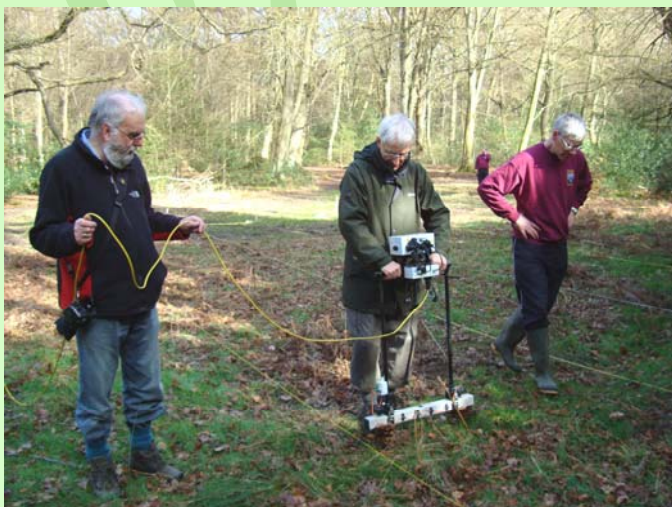
The device sends a pulse into the ground to measure the resistivity of the soil. The bottom of an ancient, filled-in ditch might be damp and therefore have a low resistivity.
